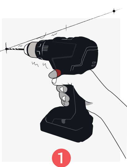
Drill holes, 3/16" diameter through drywall
